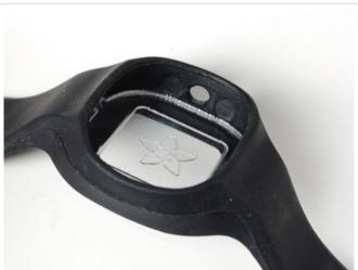
Place the clear back first into the band so it's at the bottom. Then stretch the band and scootch the assembly in, pulling the rubber to fit around!
