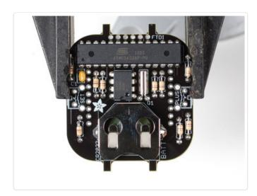
Flip it over and solder in the other battery pin, then go back and do the first one.
