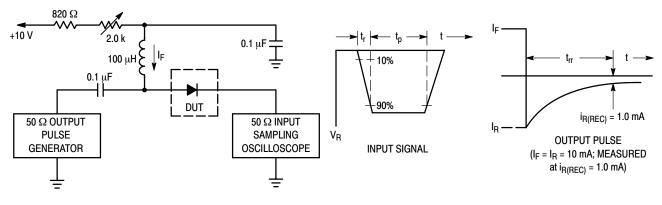
Notes: 1. A 2.0 k $\Omega$  variable resistor adjusted for a Forward Current (I<sub>F</sub>) of 10 mA. 2. Input pulse is adjusted so I<sub>R(peak)</sub> is equal to 10 mA. 3. t<sub>p</sub> » t<sub>rr</sub>
