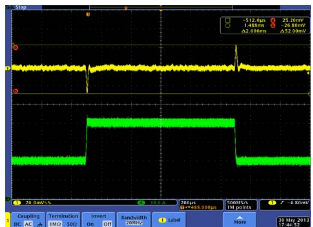
FIGURE 14. STEP RESPONSE, 20A TO 40A @ 5A/ \mu s, ASCR = 400 TOTAL DEVIATION WINDOW 50mV = 5%
